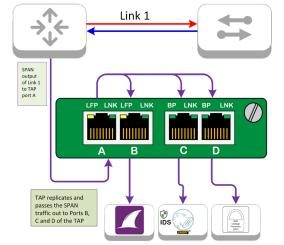
Diagram 1: SPAN port sends a mirrored output
